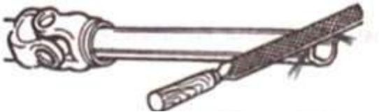
4. Shorten the equally long guard tubes to the same length as the driveline tubes.
